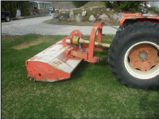
Through the work of Alvin Anderson (Manson) and *Manson Growers*, we were able to facilitate a no-cost trade for a smaller and more mobile brush shredder for the used one purchased in 2010. This smaller shredder greatly reduces the vibration and stress on the orchard tractor, as well as being much more maneuverable throughout the orchard
